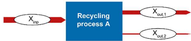
Fig. 2. Quantitative (top figure) and qualitative (bottom figure) consideration of a recycling process. Recycling process A transforms the input mass flow (left side) into two output mass flows (right side).
